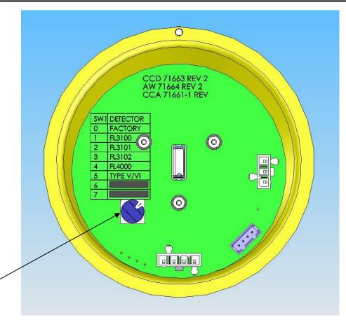
Rotary Switch shown in position 1 (for testing FL3100 Flame Detectors)
