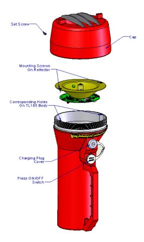
Figure 4: Reflector Mounting in Body
